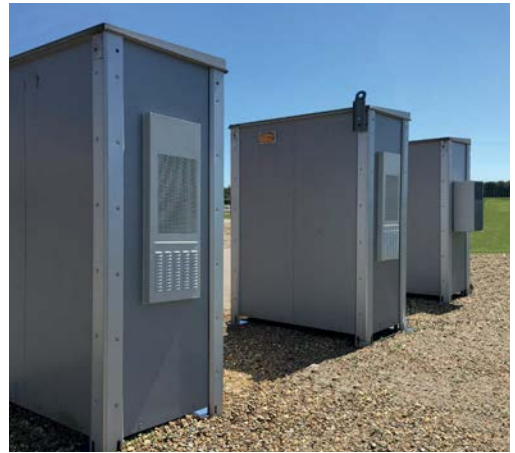
Figure 1: Test enclosures. Dimensions: 2.25*1.75*0.9m. Wall thickness: 60mm.
