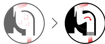
By reducing the turbulence inside the air curtain, the sound level is reduced.
