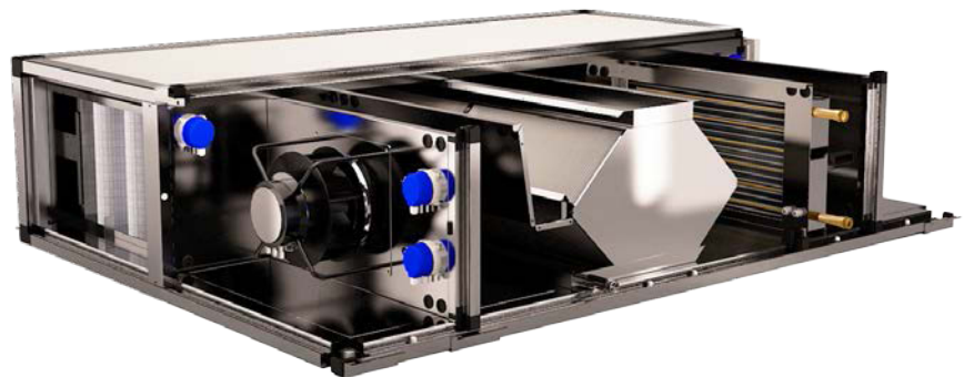
Fans of supply and extract of plug-fan-type with synchronous motor with electronic control permanent magnetos (EC)
