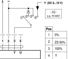
Remote control 0...100% positioner Minimum limit with positioner SG.. SG..
